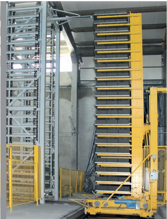
All-wheel drive automatic fingercar for increased operating speed.
