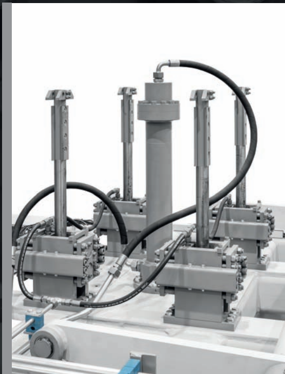
Brakes to block the tamper during demoulding.
