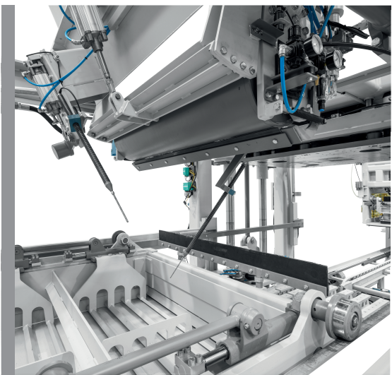
Precision filling system developed by Poyatos. Encoder controlled feeding box.
