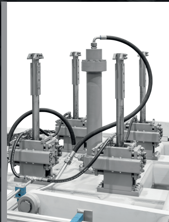
Brakes to block the tamper during demoulding.
