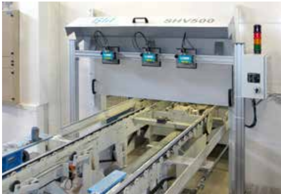
Height Control System with Chip-Reader in conveyor
